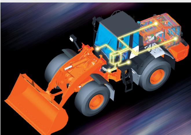
**Active Engine Control System for Digging**
