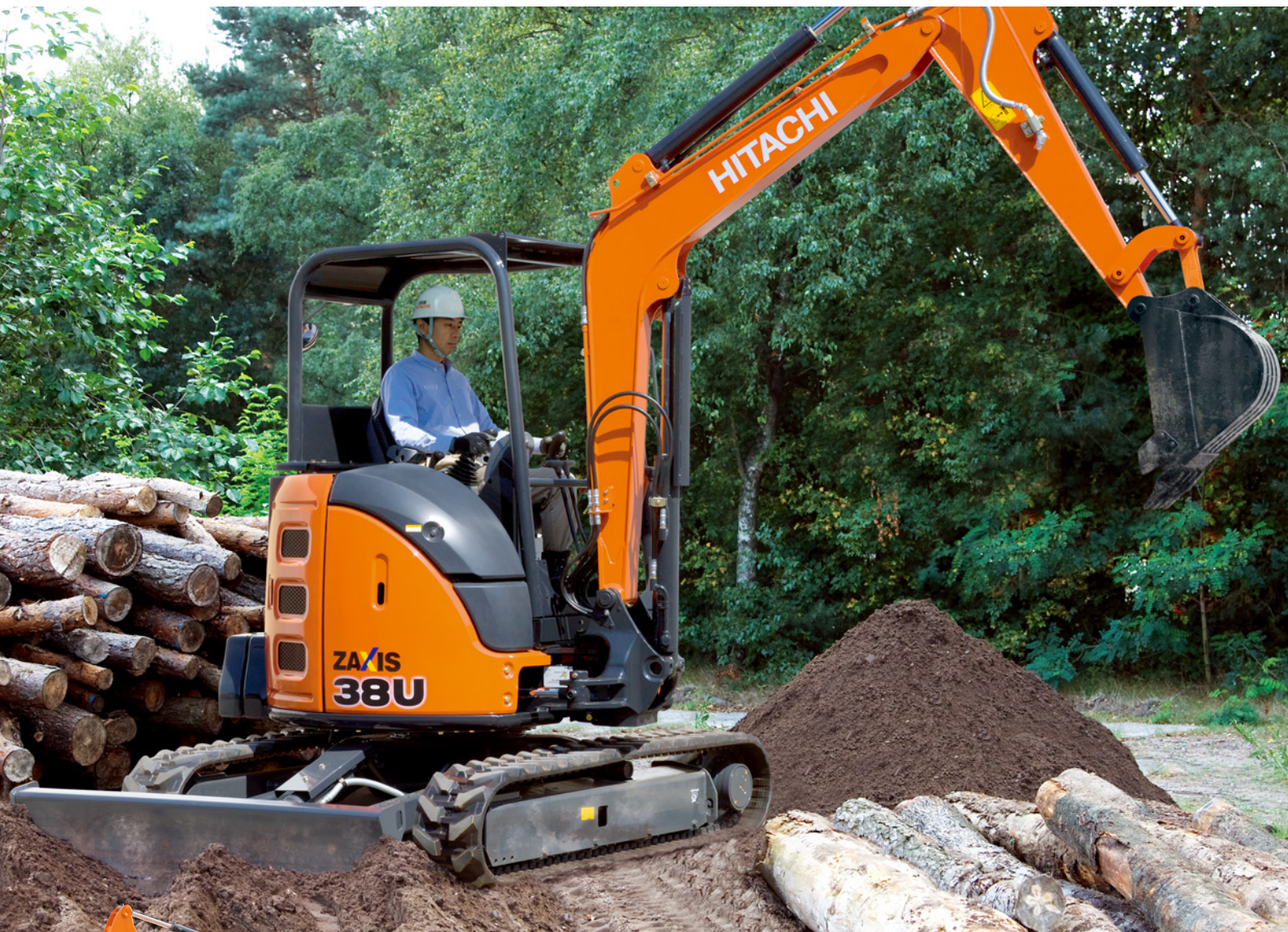
Shown equipped with 1.72 m arm, additional counterweight, armrests, extra piping and pedal as optional items.
