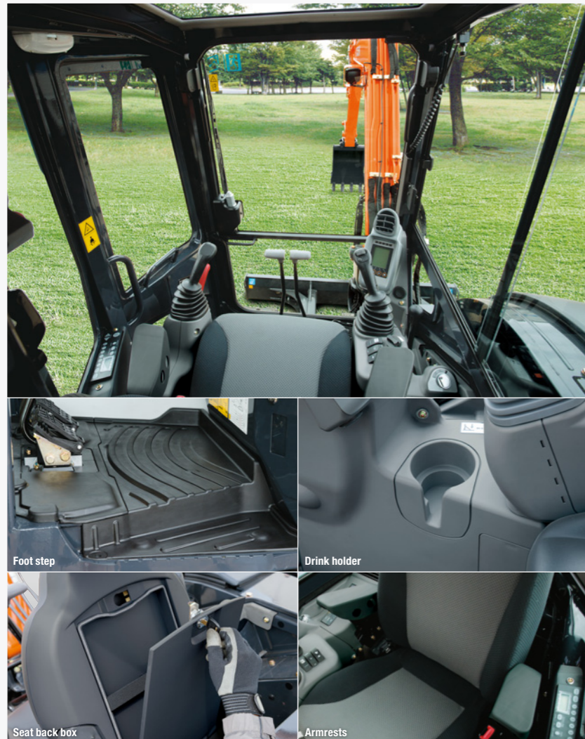
Shown equipped with cab, suspension seat, armrests, FM/AM radio, auxiliary function lever and air conditioner as optional items.
