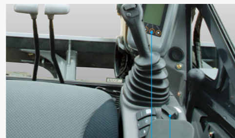
Shown equipped with auxiliary function lever and cab as optional items. ECO / PWR mode selector switch Engine control dial
