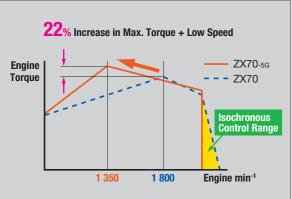
Engine torque vs. engine min-
