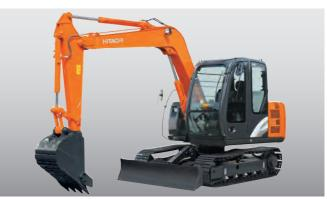
Note: The pictured ZX70 is equipped with an optional blade.
